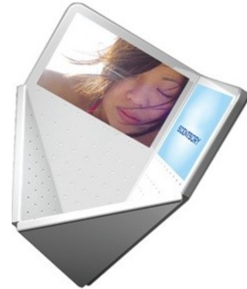
Nokia Scentsory Concept e-nose samples the odor of caller environment and transmit to recipient electronically
