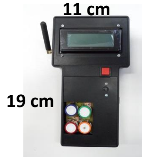
Autonomous EC Gas AQ Sensor System by ENEA, Italy
