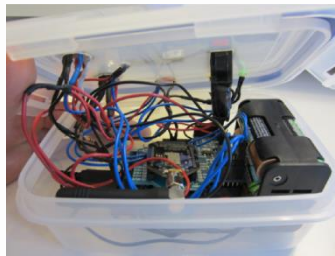
EnVisensor: Arduino-based air quality sensor module created in the frame of an MSc thesis supervised in Edinburgh University
