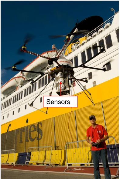
Ship exhaust plume measurement from unmanned flying platform: verification of "ship fuel" directive on sulphur in marine fuel:
