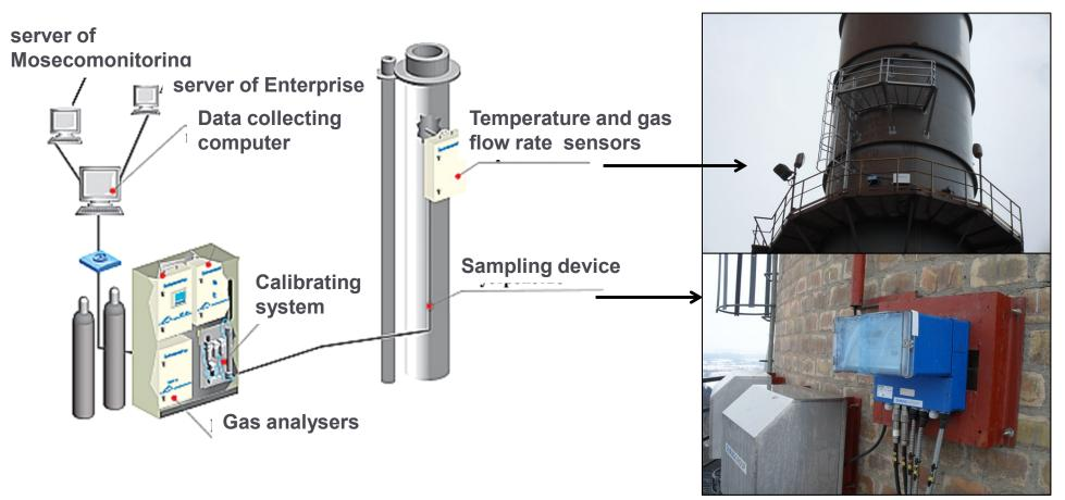
Controlled parameters: NO, NO<sub>2</sub>, CO, HCI, particulate matter, O<sub>2</sub>, temperature, gas flow rate
