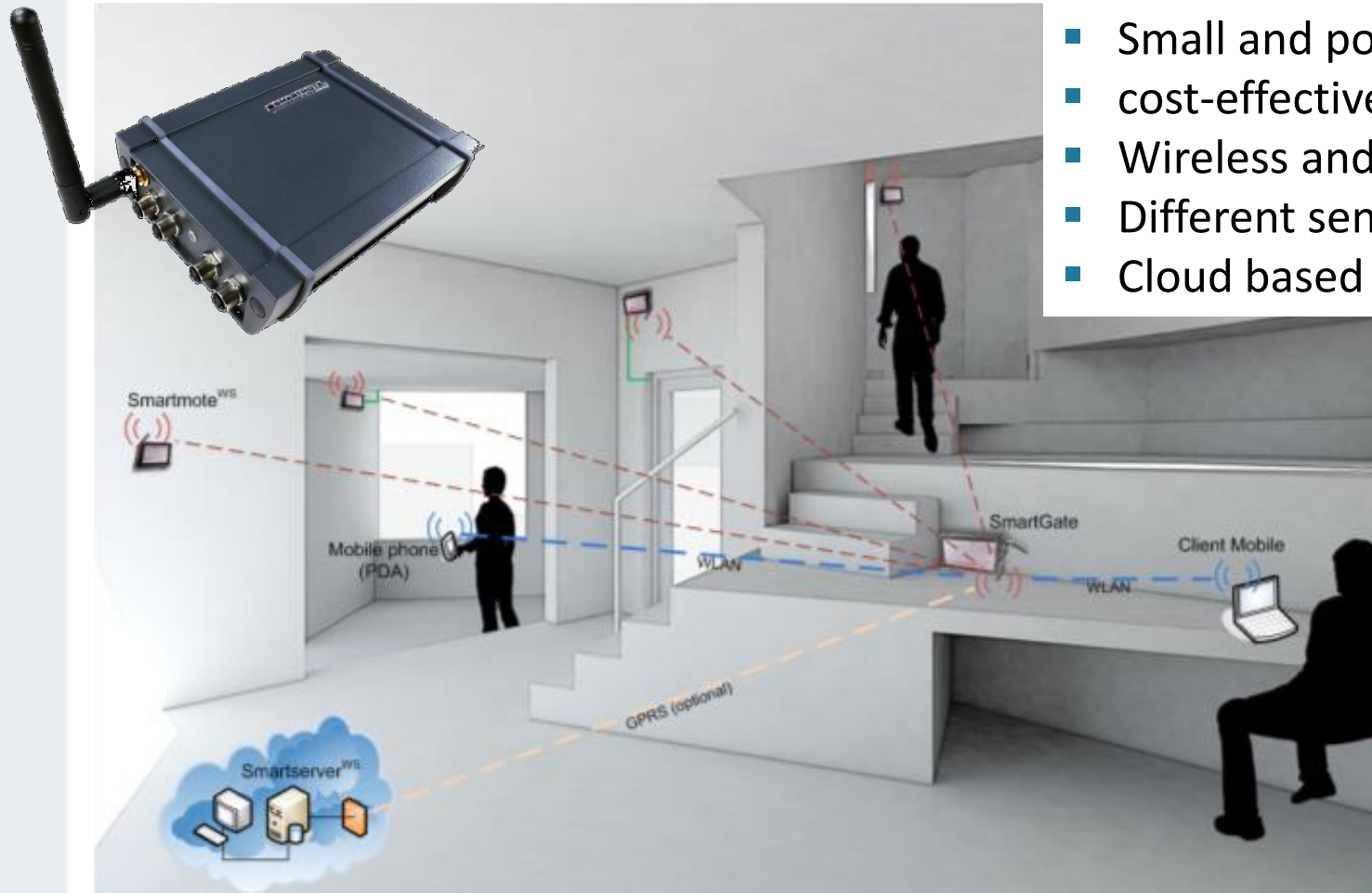
Principle sketch of a monitoring system in use (TTI Smartmote)
