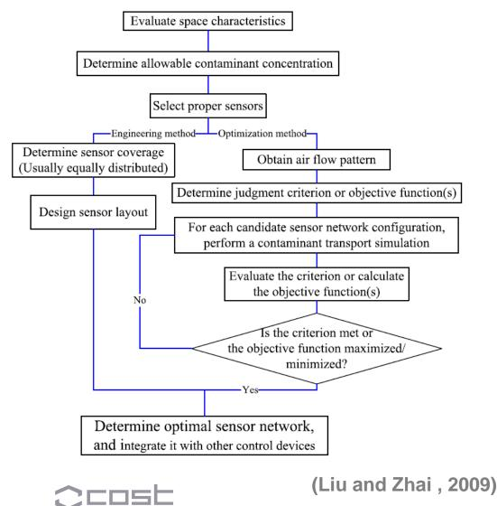
sources of pollution, ...) **Network objective** (allowable concentrations,...) **Design sensor layout** (sensor coverage, flow pattern analysis)
