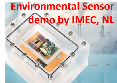
Low-ppb sensitivity for NO 2 GaN-based sensor concept
