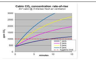
Despite normal **ventilation** the hygienic limit value is exceeded fast in a full car
