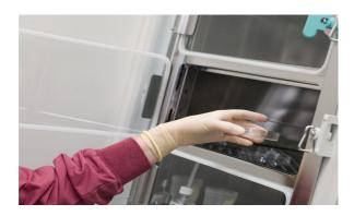
An Incubator can be described as an apparatus in which media inoculated with microorganism are cultivated at a constant temperature favourable to the growth of these microorganisms. There are big benefits by controlling the  $CO_2$  in an incubator.
