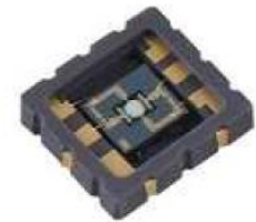
Ozone sensor chip in ceramic package Chip size 1.7 x 1.9 mm Package size 5 x 5 mm
